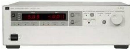
Figure D.5: HP 6035A power supply.
